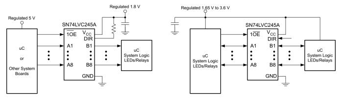
Figure 4. Typical Application Schematic
