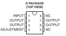
NC No internal connection OUTPUT terminals are all internally connected.
