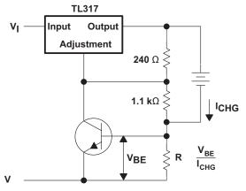
Figure 7. 50-mA Constant-Current Battery-Charger Circuit
