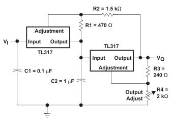
Figure 5. Tracking Preregulator Circuit
