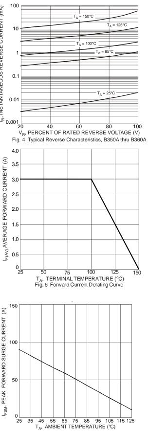
Fig. 8 Non-Repetitive Forward Surge Current Derating Curve
