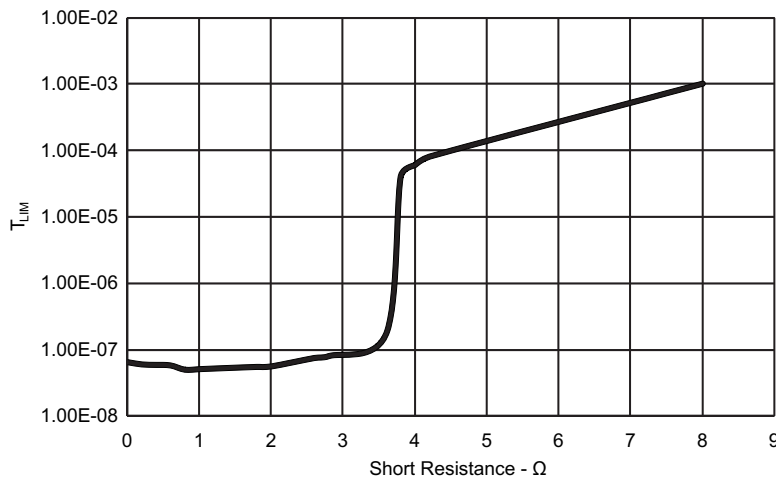
Figure 11. Overcurrent Response Time vs Short Resistance
