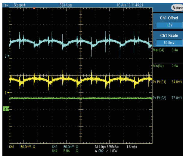
Figure 10. Ripple for Buck 1 (Yellow Trace) 1.2 V, 3 A and Buck 2 (Blue Trace) 1.8 V, 2 A, 50 mV per Division V_{IN} = 12\text{ V} , f_{SW} = 500\text{ kHz} , L_O = 4.7\text{ }\mu\text{H} , \text{DCR} = 10\text{ m}\Omega , C_O = 22\text{ }\mu\text{F}
