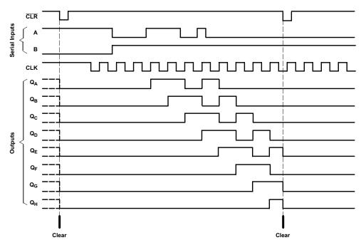
Figure 1. SN74HC164 Example Timing Diagram
