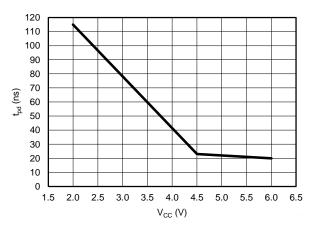
Figure 5. Propagation Delay vs Supply Voltage at T<sub>A</sub> = 25°C
