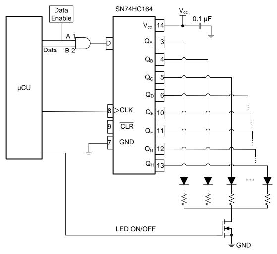
Figure 4. Typical Application Diagram
