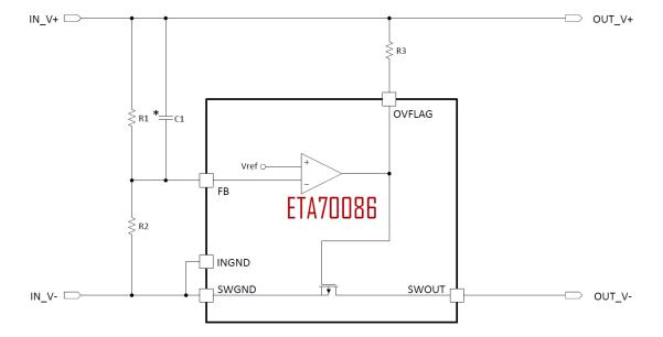
\* R1 can be replaced by a Zener Diode
