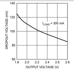
Figure 5. Dropout Voltage
