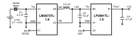
Figure 19. LP3991 Used as a Post DC-DC Regulator
