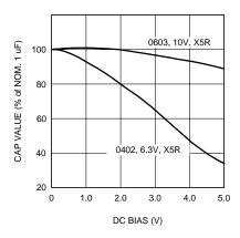
Figure 13. Effect of DC Bias on Capacitance Value
