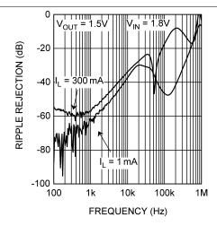
Figure 10. Power Supply Rejection Ratio
