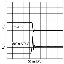
Figure 8. Short Circuit Current
