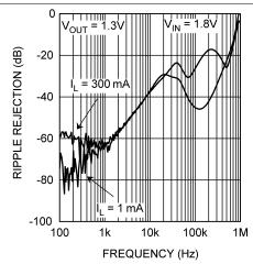
Figure 9. Power Supply Rejection Ratio
