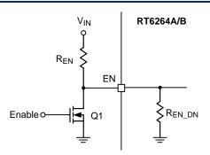
Figure 8. Digital Enable Control Circuit
