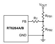
Figure 2. Output Voltage Setting
