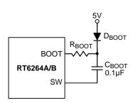
Figure 12. External Bootstrap Diode and Resistor at the BOOT Pin
