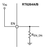
Figure 6. Automatic Start-Up Setting
