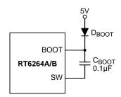
Figure 10. External Bootstrap Diode
