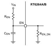
Figure 7. External Timing Control
