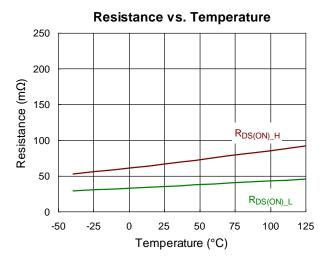
Figure 13. RT6264A/B RDS(ON) vs. Temperature
